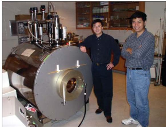
Xiaoping Hu (left) and CBN post-doc Xiaodong Zhang have adapted the small animal MRI scanner at the Emory School of Medicine to image the crayfish brain. Currently, they are working to enhance the resolution of the scanner and develop a customized coil for the crayfish head.
